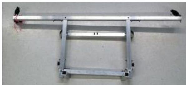
Figure 8: Tiller strut that leads lines from the levers to the tiller
