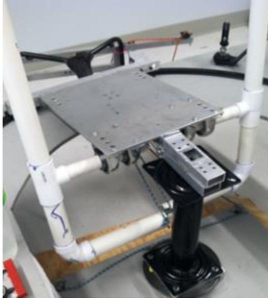
Figure 4: Lever arms used to move the tiller in the Skipper's Chair. Design based off combination of crank mechanism and tractor seat.
