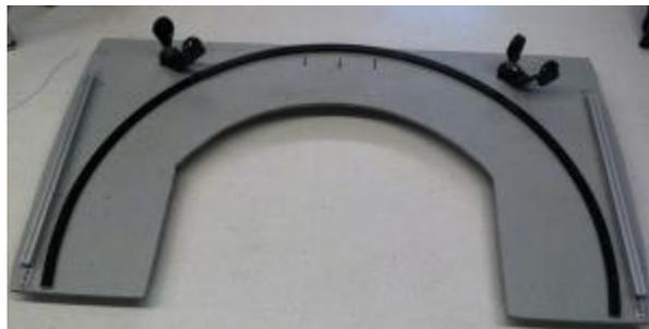
Figure 5: Rounded track used to move the skipper from port to starboard
