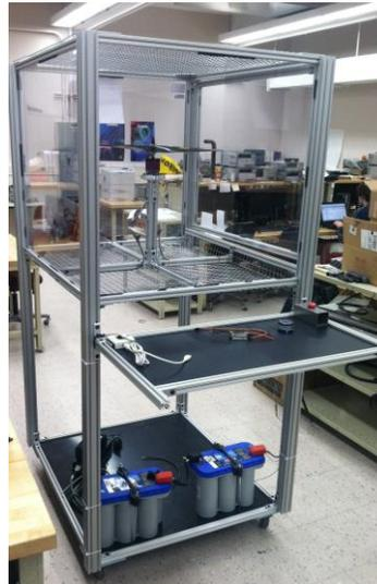
Figure 2: Final Design of Thrust Module
