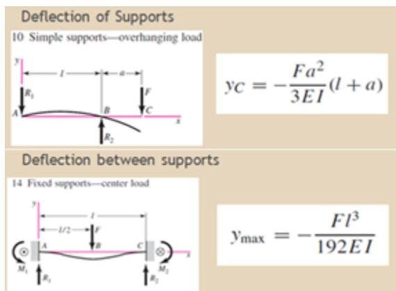
**Figure 2 – Deckloo Structural Analysis**
