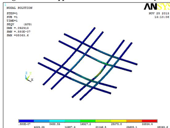
Figure 5 - Rebar ANSYS Analysis
