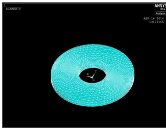
Figure 1: ANSYS Slab Model Mesh Area
