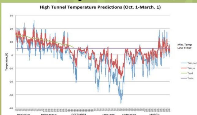
Using data that depicts the weather patterns of Rochester, NY for a typical Meteorological year, the concepts of heat transfer and thermodynamics were applied to create a thermodynamic model that allows us to predict the thermal behavior of the system and accurately estimate heating needs for the winter season.
