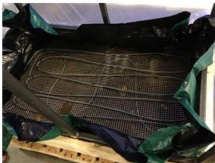
Picture 2: Heating Coils in Test Facility Before Covered in Soil
