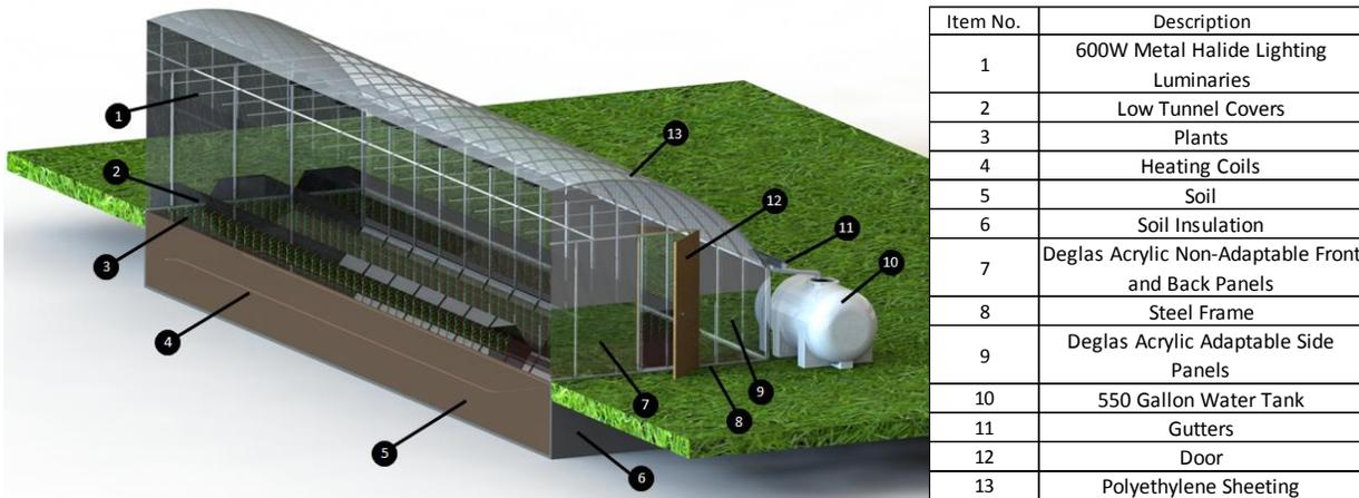
Figure 3: Cutaway of Final High Tunnel Design with Feature List
