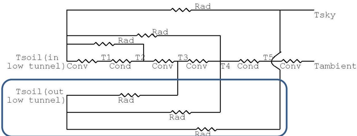
Figure 6: Thermal Circuit of the High Tunnel
