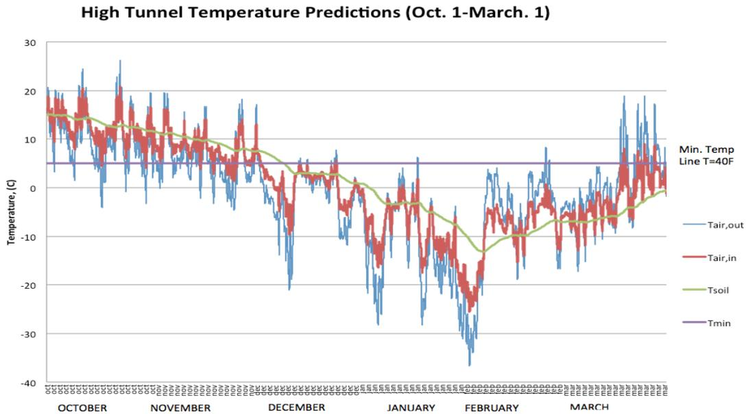
Figure 7: High Tunnel Temperature Simulation- Current State
