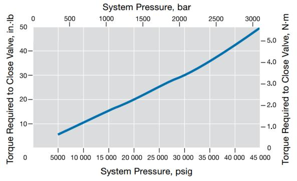
This plot shows opening torque versus system pressure. At 10000 psi, the opening torque is roughly 175 oz-in, which is equal to the output of our stepper motor.
