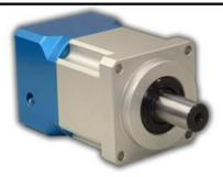
The 3:1 ratio increased the step resolution from 1.8 degrees to .6 degrees. Also increased was the torque output, which increased from 175 to 525 oz-inches. Both the output torque and step resolution are important for the control of the valve. A
