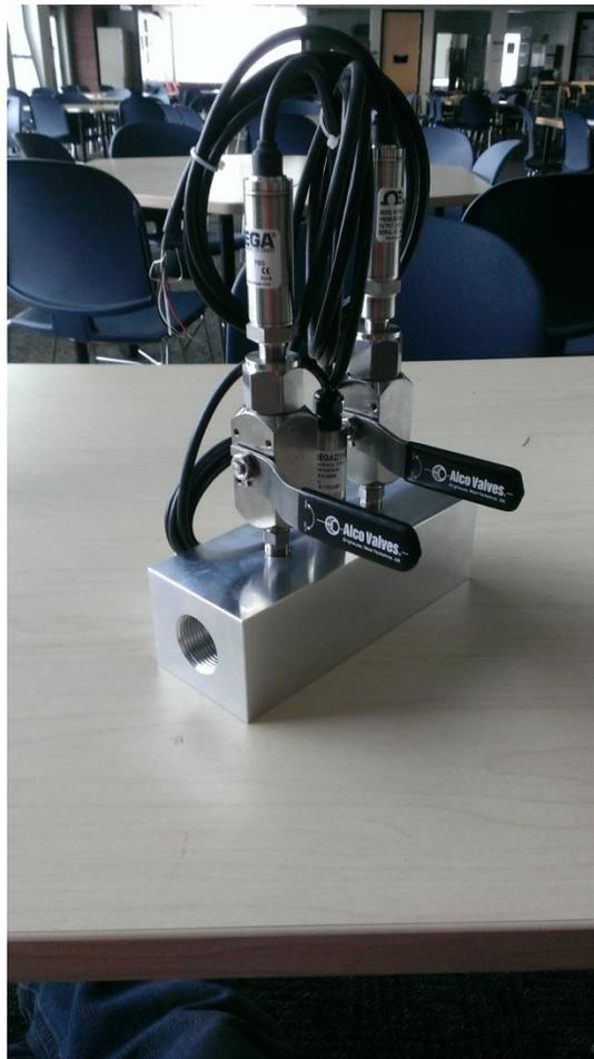
Figure 2: Assembled Pressure Transducer Manifold
