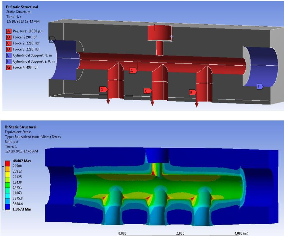
To help eliminate the risk of failure, we identified the major failure modes possible with our design and tried to identify a recommended action to reduce each.
