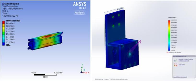
**Figure 11. Example Finite Element Analysis conducted to determine deflection under loading for key system components. Left is deflection of a motion rail and right is deflection of the EMHI.**
