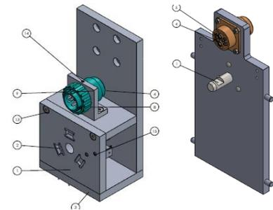
Figure 5. EMHI (left) and UMB (right) Subsystem CAD Models.
