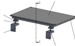
Figure 10. Bed CAD model. Two of the three leveling feet are visible.
