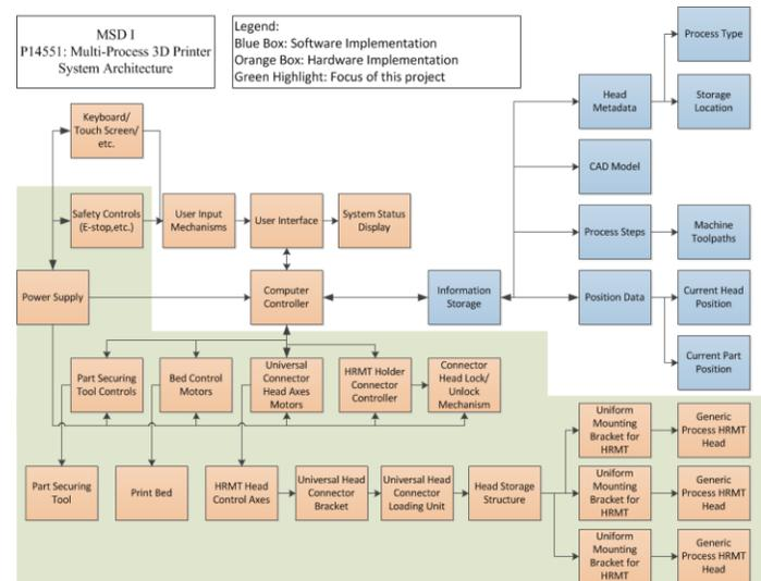
**Figure 1. System Architecture diagram identifying key hardware (orange) and software (blue) elements of the system. System components identified as within the scope of this project are highlighted in green.**
