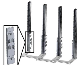
Figure 7. Storage system with storage bracket detail CAD Model.
