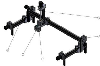
Figure 6. Three-axis motion system CAD Model.
