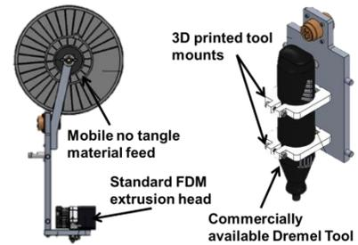
Figure 9. CAD models of two implemented process heads with added callouts.
