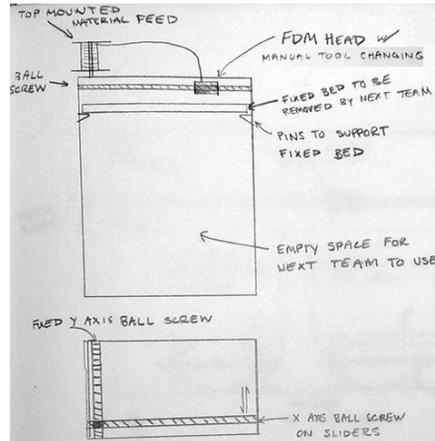
Figure 3. Pugh Matrix Concept Two: A two-axis FDM with rudimentary system design elements.
