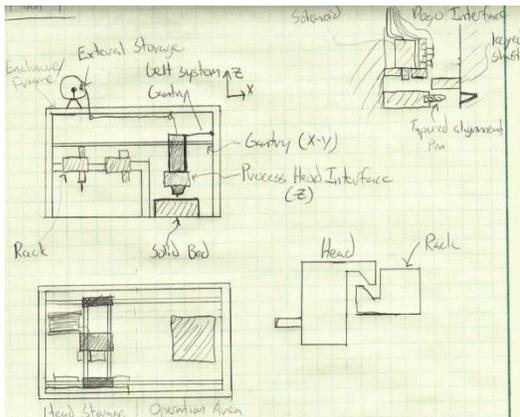
Figure 4. Pugh Matrix Concept Seven: A planar gantry system with vertical movement controlled by a vertical element mounted to the gantry.
