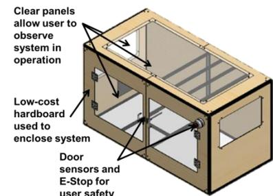
Figure 8. System enclosure CAD model with identified system elements.
