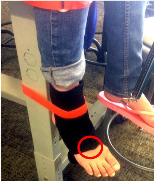
**Figure 1:** Setup #1, fishing line attached at end of brace (see circled area).
