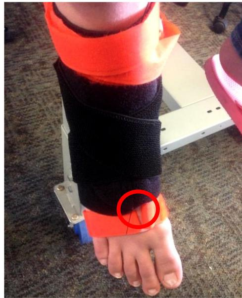
**Figure 2:** Setup #2, fishing line attached to the Velcro strap that is tied to the ankle brace (see circled area).
