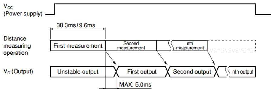
From this information, worst case to first output would be 53ms. This is assuming that operation has stabilized (meaning that power has been applied at least 100ms previously).
