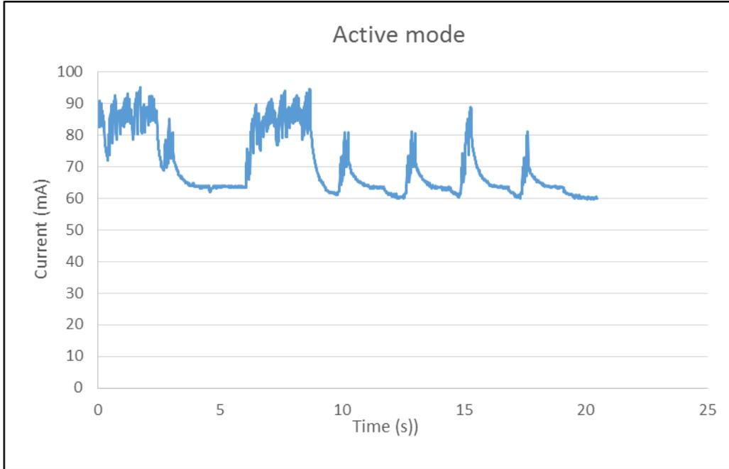
Figure 1: The following plot displays the raw data which represents amount of current that is drawn when the dive is being used in active mode. Each spike represents heel strike
