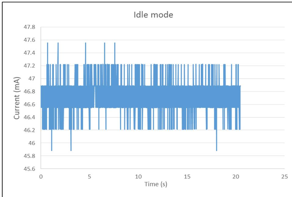
Figure 2: The following plot displays the raw data of current drawn when the device is in idle mode. No steps taken
