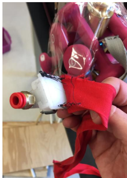
Muscle base and red inelastic ribbon after failure
