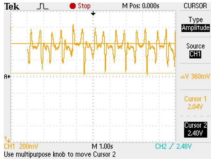
**Figure 3. Analog Output Voltage of the accelerometer undergoing sweeping motion**
