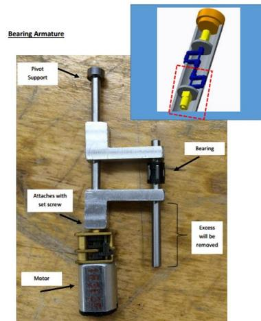
Figure 1. Bearing armature for cane handle
