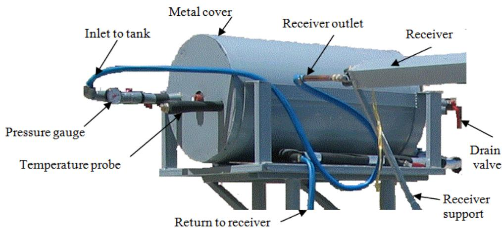
Figure 4: Thermal storage tank configuration.
