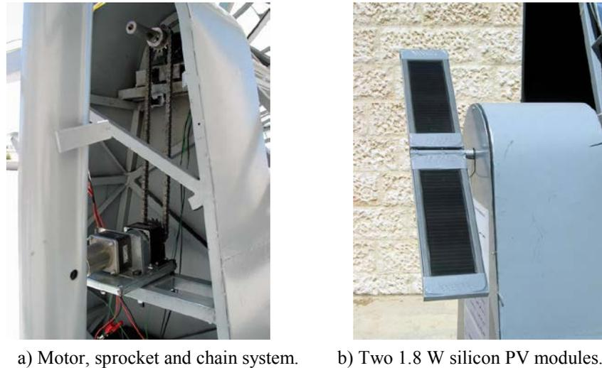
Figure 5: Tracking motor mechanism with a PV power unit mounted on a tracking shaft.
