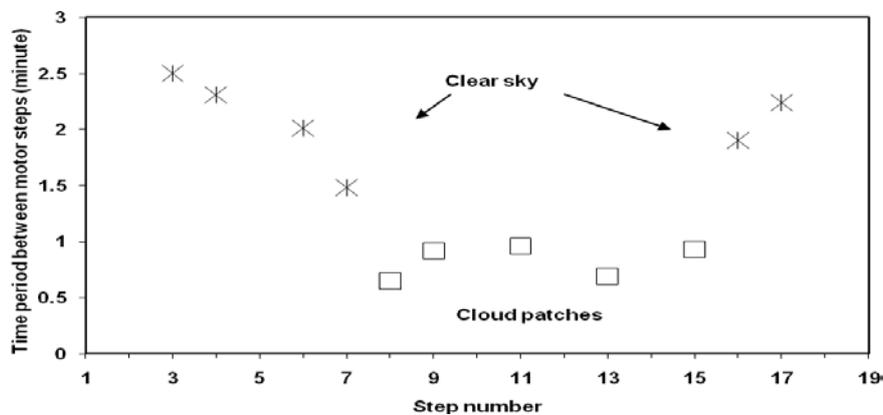
Figure 9: Solar tracking sensitivity during a cloudy day.
