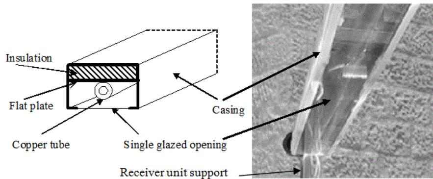
Figure 3: Flat receiver configuration.
