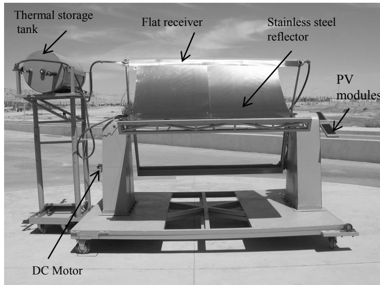
Figure 7: Test platform operating in a sunny day.
