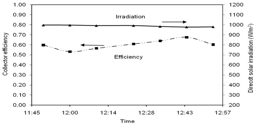
Figure 8: Collector performance during noon hour, working fluid is water,  $\dot{m}_w = 0.0233$  kg/s, N-S tracking axis.
