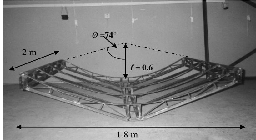
Figure 2: Parabolic steel frame.
