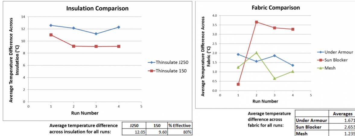
**Figure 5: Temperature difference across the various insulations (left) and fabrics (right).**
