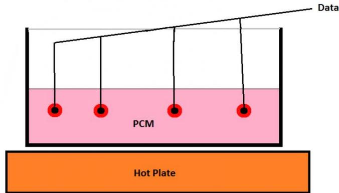
**Figure 2: PCM Properties Test Set-up**
