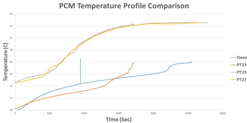
**Figure 3: Plot of the PCM temperature profiles while undergoing the PCM properties test.**
