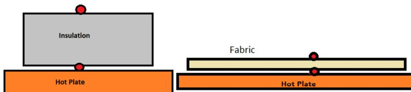
**Figure 4: Insulation (left) and fabric (right) test set-ups consisting of the hotplate, temperature sensors, and either insulation or fabric.**
