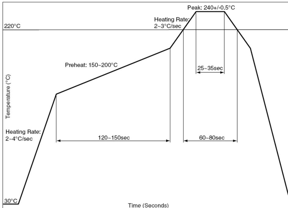
The reflow profile shown above should not be exceeded, since excessive temperatures or transport times during reflow can damage the module. Cooling temperature fall rate: max 3°C / sec
