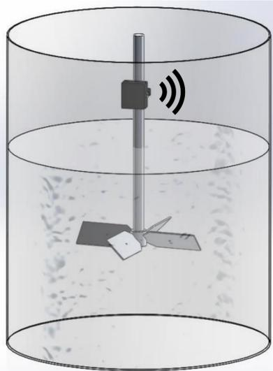
The overall setup was designed around the test tank provided by SPX. Wires run from the enclosed telemetry system (box at the top of the shaft), down the shaft to the four strain gauges. The wire as well as its connections must be waterproofed, allowing for data to be safely and accurately transmitted. The strain gauges must also be waterproof, and they were covered with epoxy after mounting in order to ensure water protection.
