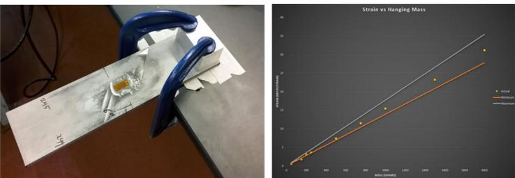
Evident by the plot to the right of our setup, measured strain for this setup falls between the expected range of strain calculated using beam bending equations with material tolerances taken into consideration.
