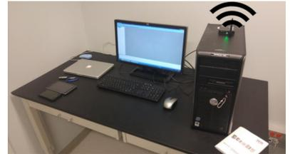
Once the transmitter receives data from the strain gauges, it transfers it to a nearby computer over the 2.4 GHz spectrum (Wi-Fi). This data can then be imported to Matlab or Excel for processing and analysis.
