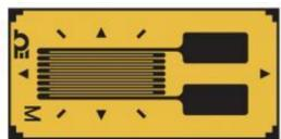
Linear strain gauges were chosen due to their sensitivity to the small changes in strain that will be seen during impeller blade operation.
