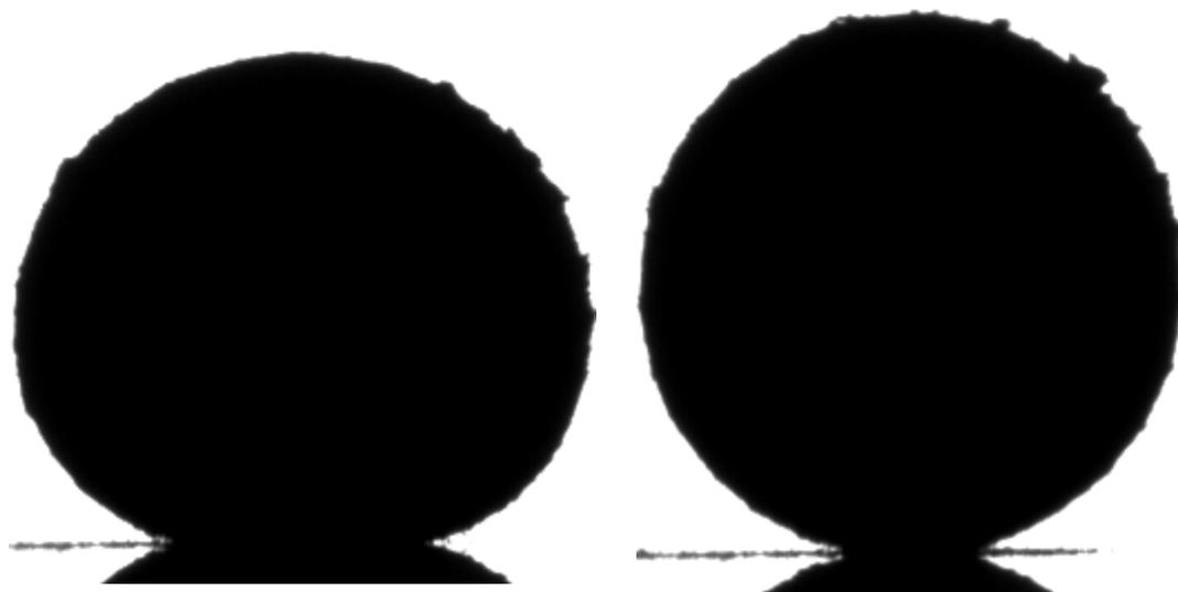
Figure 2. Marble shapes in the absence of electric field (A) and under electric field of 21 cgse (B).
