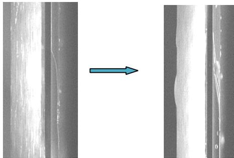
(a) The groove depth is 0.2 mm, the groove width is 0.6mm
