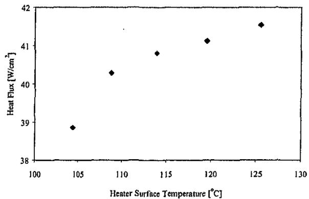
Figure 7: Heat transfer characteristics of a simple water-filled VIDA cell
