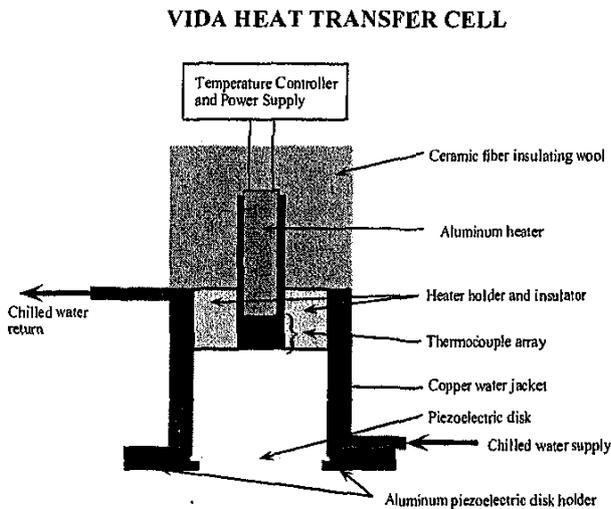
Figure 6: VIDA heat transfer cell with water jacket
