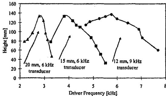
Figure 4: Maximum projection height of droplets as a function of driver frequency
