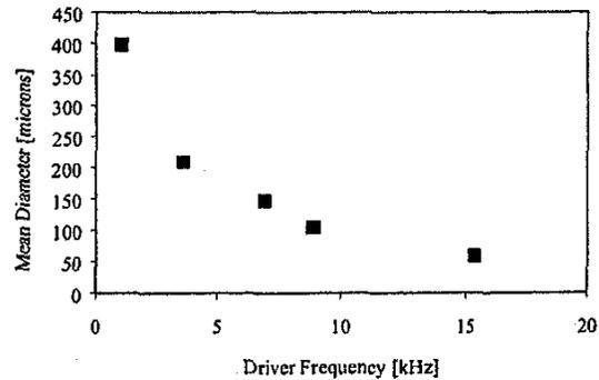
Figure 5: Secondary droplet mean diameter as a function of driver frequency
