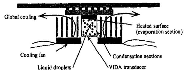
Figure 1: VIDA heat transfer cell with external fins and fans
