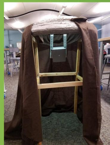
Simulate pit setup used to test the counting system
