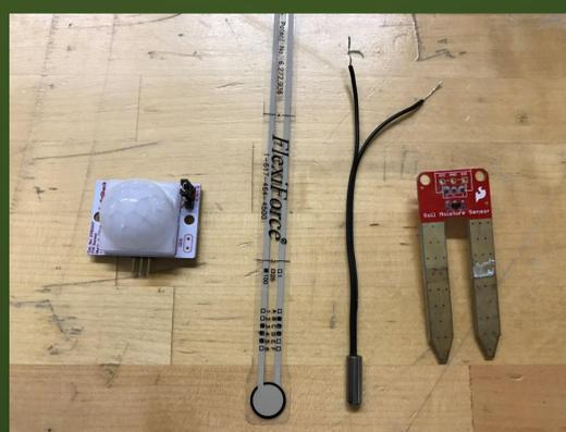
From left to right: motion sensor, pressure sensor, temperature sensor, soil moisture sensor
