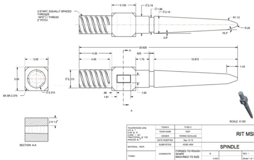
Figure 4: Drawing of the spindle.
