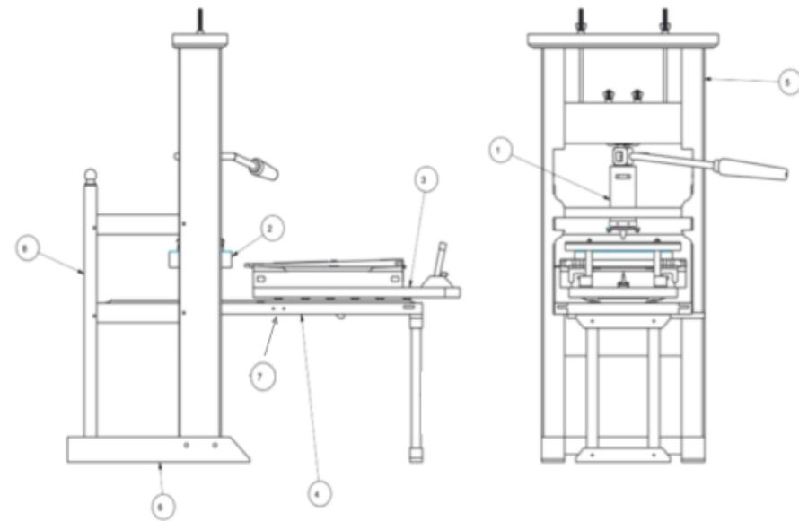
Figure 2: Assembly drawing of press.
