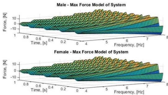
Figure 6. Max force curve along the hand simulation results assuming uniform mass distribution over 1 unit of time for a 240 lbs human.
