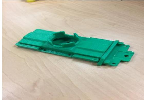
Figure 4. 3D printed brake chassis/skeleton.
