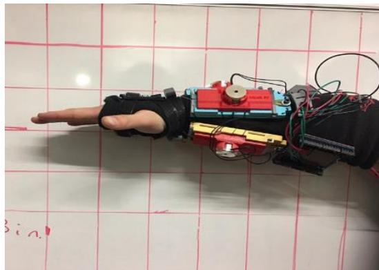
Figure 5. Overall glove integration mapped against an inch by inch grid
