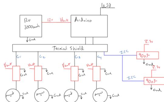
Figure 8. Beta Block Diagram
