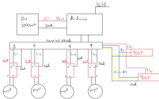
Figure 9. Beta Wiring Diagram
