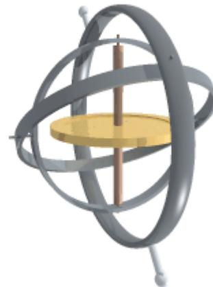
The GyroGlove uses a gyroscope not unlike the control moment gyroscope used on the International Space Station, the one that allows it to pivot in space without using fuel. It's simple, easy to manufacture, and it can be made very small. This low-overhead application is why the GyroGlove's power pack can be so thin and light: it doesn't require a big battery to do what it does.
