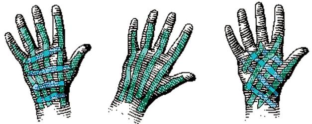
Figure 2 Piezoelectric fibre composite placement in glove structures.
