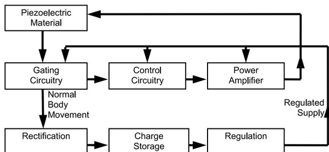
Figure 3 Active vibration suppression and energy harvesting circuit.
