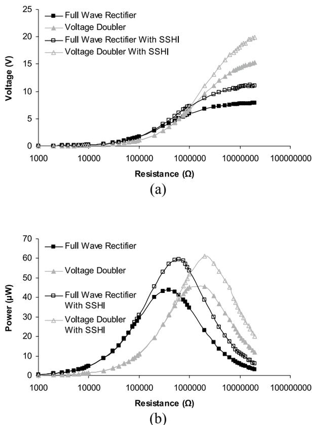
Figure 5 Comparison of PFCs in terms of (a) voltage and (b) power, with and without the semi-active damping technique.
