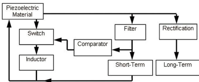
Figure 4 Semi-active vibration suppression and energy harvesting circuit.
