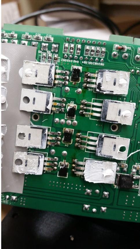
The question now becomes, why were the transistors shorted? After looking at various sources online and documentation for the MA860H, it seems that the MA860H was expecting active low pulses while the Arduino was providing active high pulses. This is a problem.
