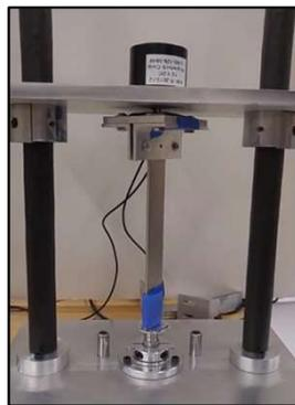
Final Structure Levitating Clamp and Test Coupon
