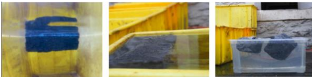
Biochar lime blocks are so light they float!
