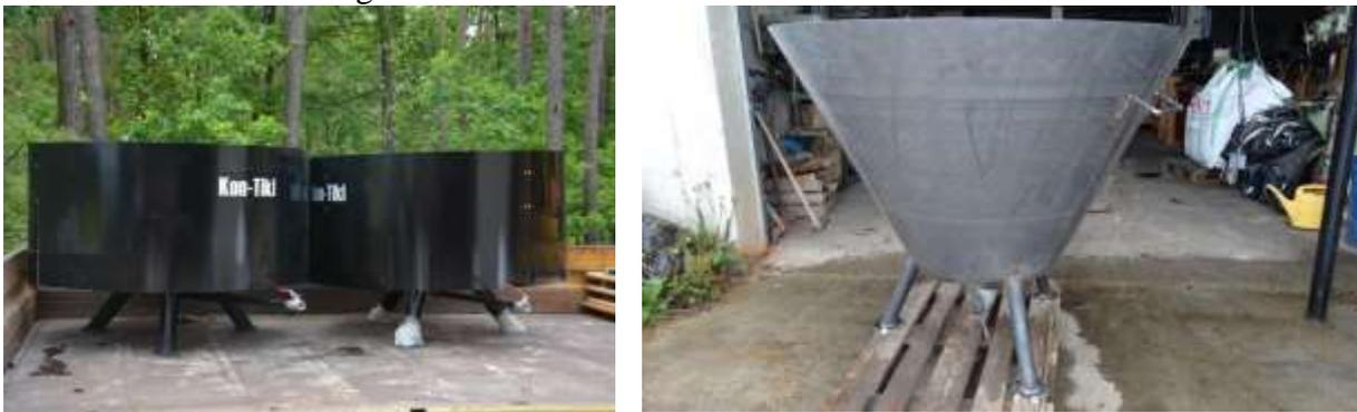
**Figure 1: The Kon Tiki with and without its heat shield**
