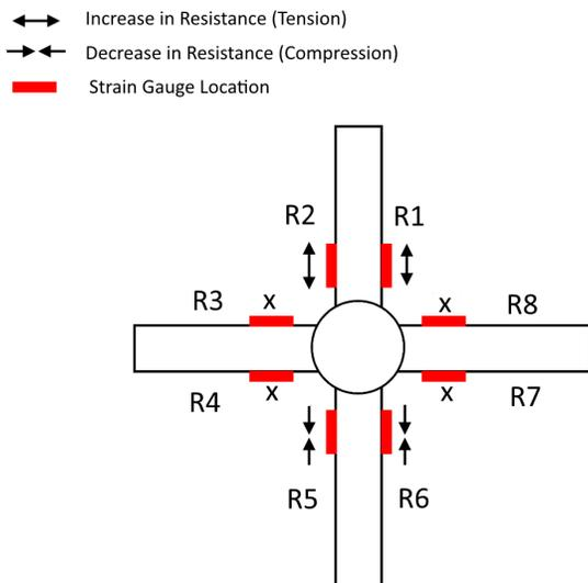
Figure 1: Structure Layout (Bending Moment)
