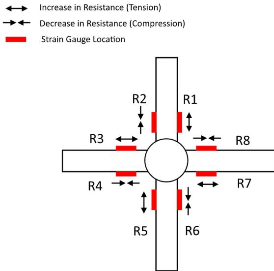
Figure 3: Structure Layout (Torsional Load)
