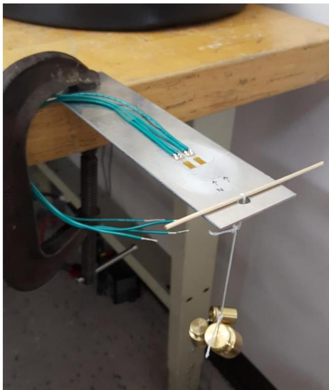
Figure 5: Cantilever Beam Test
