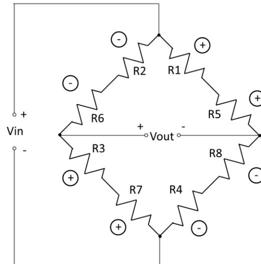
Figure 4: Wheatstone Layout (Torsional Load)
