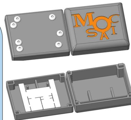
Figure 3: The 3D model of the housing that integrates with the shirt iteration. The microcontroller is soldered onto metal snaps in the housing which contact the snaps sewn into the shirt. The snaps in the shirt are connected to the electrodes with conductive thread.
