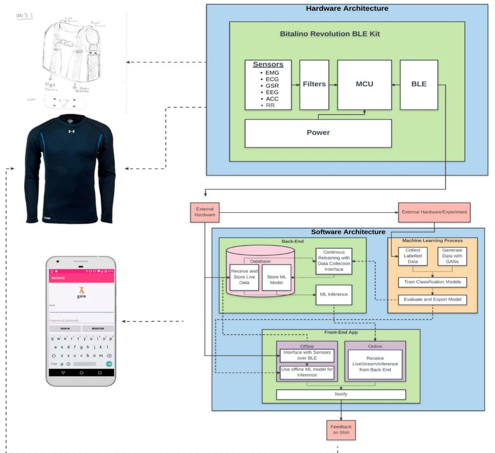
Figure 1: Operations flow of the hardware and the software architecture (above).
