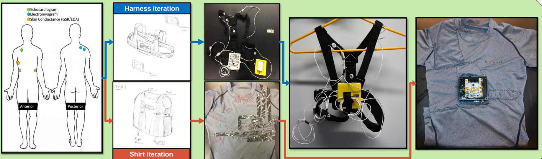
Figure 2: Diagram of electrode placement on the surface of the skin. Concept drawings of the harness and shirt iterations. Pictures of the build progress. Pictures of the final designs of both iterations of prototype.
