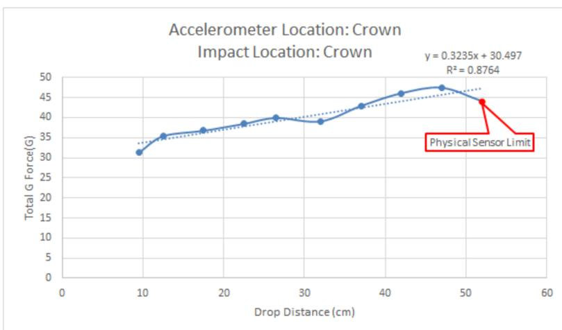
Fig 5: Impact Testing Data
