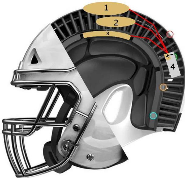
Figure 9: Possible Sensor Placements. 1 - outside, 2 - inside padding, 3 - around head, 4 - large battery placement
