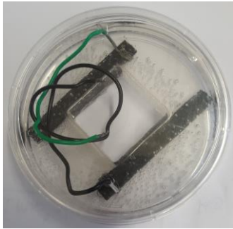
Bailey's Prototype: Petridish with electrodes at opposite end of the dish held in place by silicone
