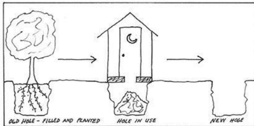
**Figure 1: Schematic of the working logistics of an arborloo.**
