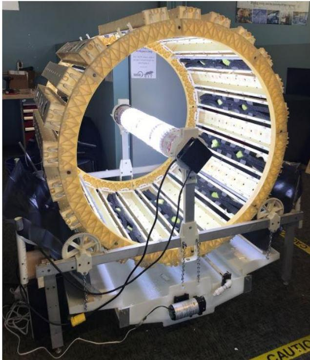
Figure 8. Fully assembled, working Surculus with crops.
