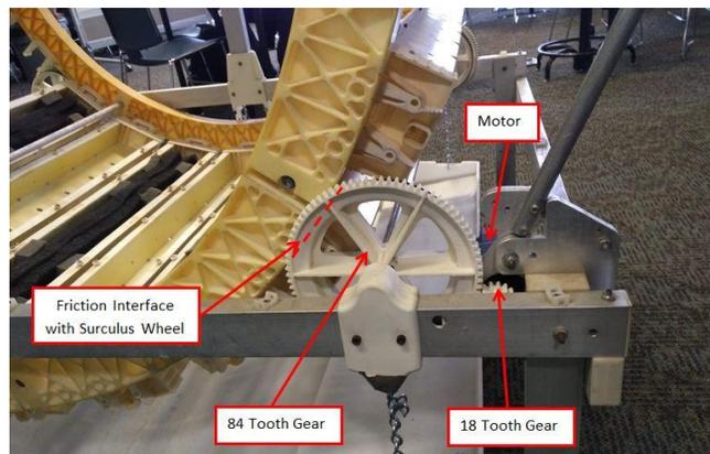
Figure 5. Motor and gear configuration for the Surculus.
