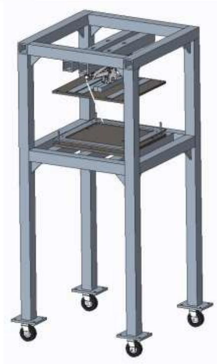
Figure 4: Final Assembly Model of Plastic Melting and Compression System
