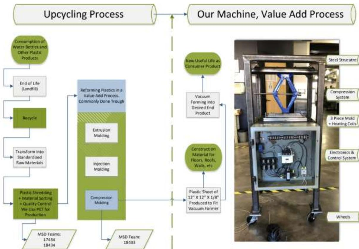
Figure 1: Upcycling Process Flowchart
