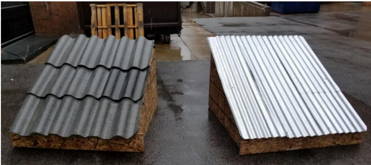
**Team P1748's Roof Design being compared to standard galvanized roofing in the rain.**
