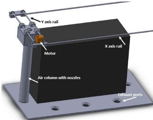
**Figure 1:** Rail system around computer
