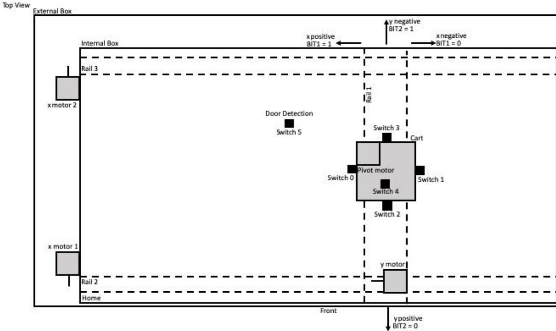
**Figure 6: Motor and Switch Designation Drawing**
