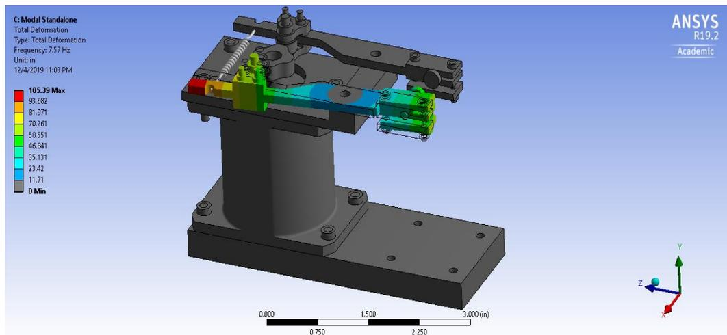
Figure 3. Results from modal analysis showing the first mode of 7.95 Hz.
