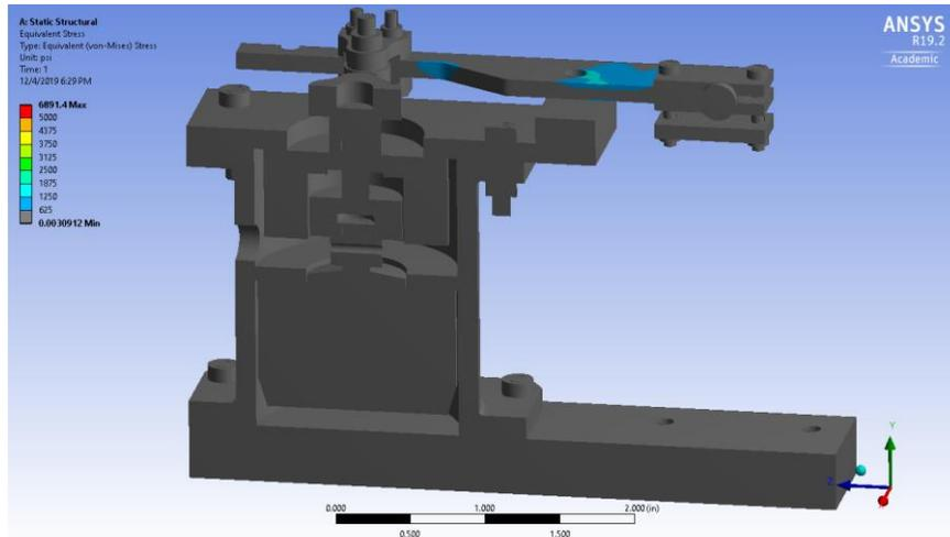
Figure 1. Results of static structural analysis showing equivalent (Von Mises) stress
