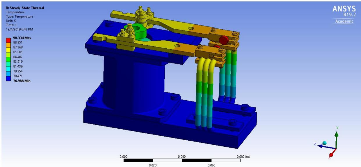
Figure 2. Plot of temperature from ANSYS thermal analysis run at 77K baseplate temperature.
