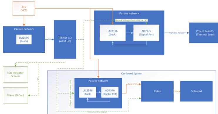
Figure 1: Lab test system PCB Block Diagram
