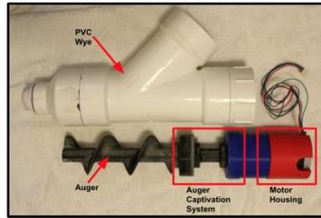
Figure 3: PVC Wye, Auger, and Stepper Motor in Housing
