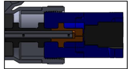
Figure 4: Cross-section view of Extruder Motor Housing and ACS
