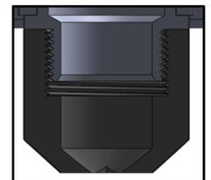
Figure 6: Section view of the extruders nozzle.
