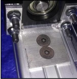
Figure 10: Ball Screw Support Block Bracket
