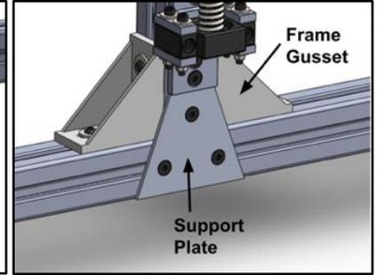
Figure 13: Z-Axis, Z-motor Support and Frame Gusset
