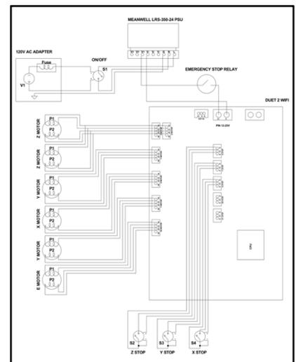
Figure 18: Electrical System Schematic
