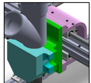
Figure 9: Extruder Mount in Printer
