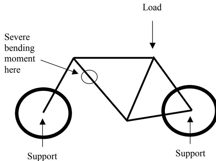
**Figure 1:** Forces acting on a typical bicycle frame
