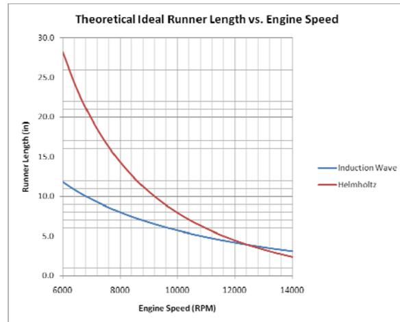
Figure 3. Theoretical Runner Length V. Engine Speed
