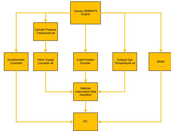
Figure 13. Dynamometer Electrical Test Diagram
