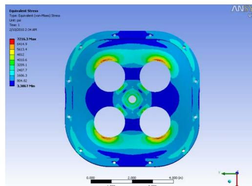
Figure 9. Static Analysis of Plenum Base
