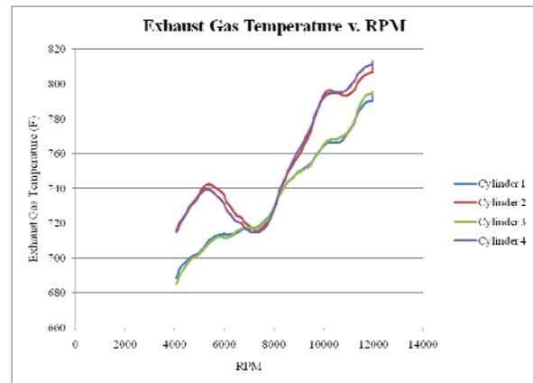
Figure 14. Exhaust Gas Temperatures for Current Engine
