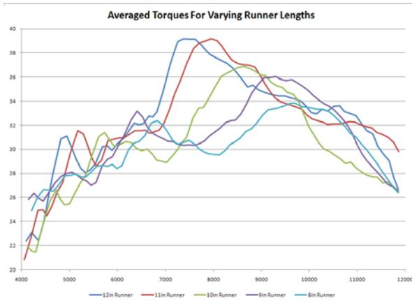
Figure 4. Average Torques for Varying Runners Lengths
