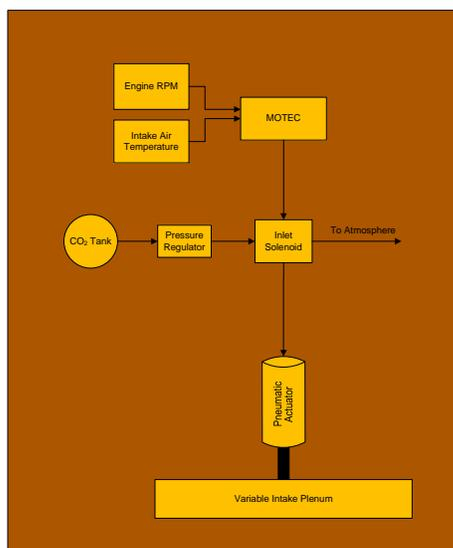
Figure 10. Electro-Pneumatic Actuation Block Diagram
