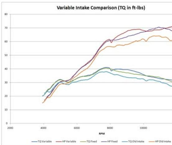
Figure 12. Comparison of Variable to Static Intake Horsepower and Torque
