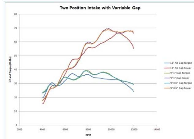
Figure 5. Resulting Horsepower and Torque of Test Two Position Intake with Varying Gap Width
