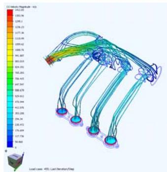
Figure 2. Air Flow Path Results from CFD Analysis
